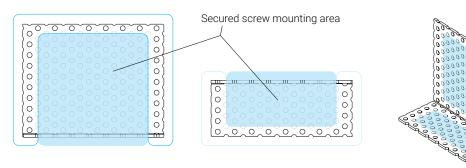
Do not try to drill holes or nails through the outermost holes when installing the screws on the bracket.
