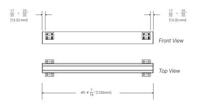
Use this dimension for drilling holes to install brackets and screws.
