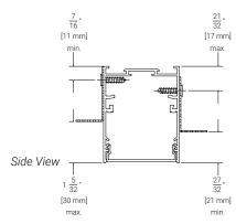
Use this dimension to determine the thickness of the dry wall or wood panel.
