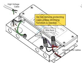
Twist the same color cables on together by wire nuts to connect the 24V cables.
