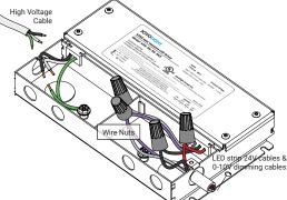
Twist the same color cables on together by wire nuts to connect the 24V cables.
