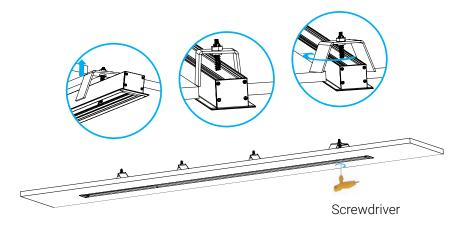
**STEP 4** 1. Stick the LED tape on 2. Assembling the lens cover.
